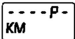
Oil pressure failure detection
