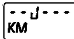
Gauge failure detection
