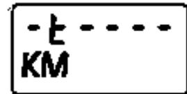
Oil temperature failure detection
