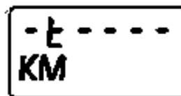
Oil temperature failure detection
