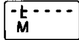
Oil temperature failure detection
