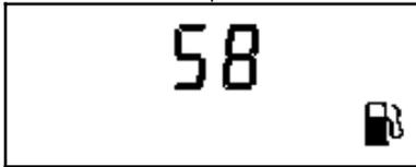
Maximum fuel level displayed when the tank is not full.
