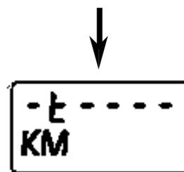
Oil temperature failure detection
