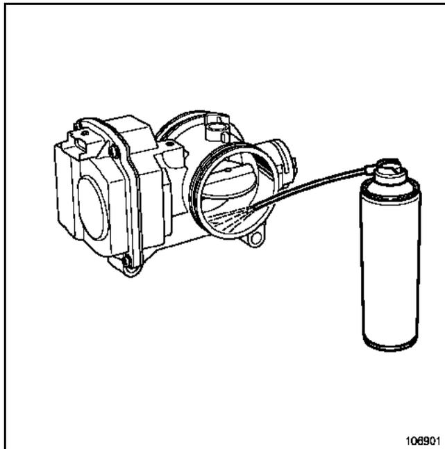
Hold the throttle valve flap open manually.
