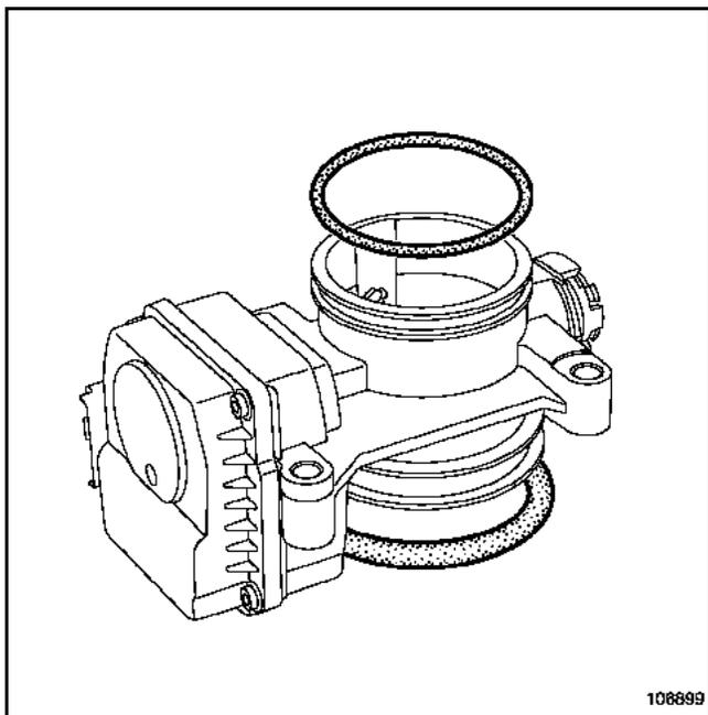
Remove the external O-ring seals from the throttle valve.
