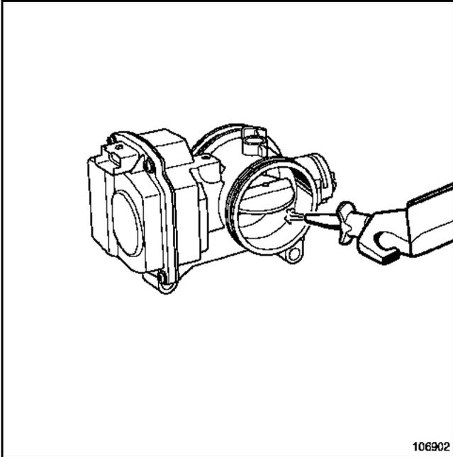
Blow out any paper debris with compressed air from the nozzle. Blow first around the valve, then inside the throttle valve cavity.
