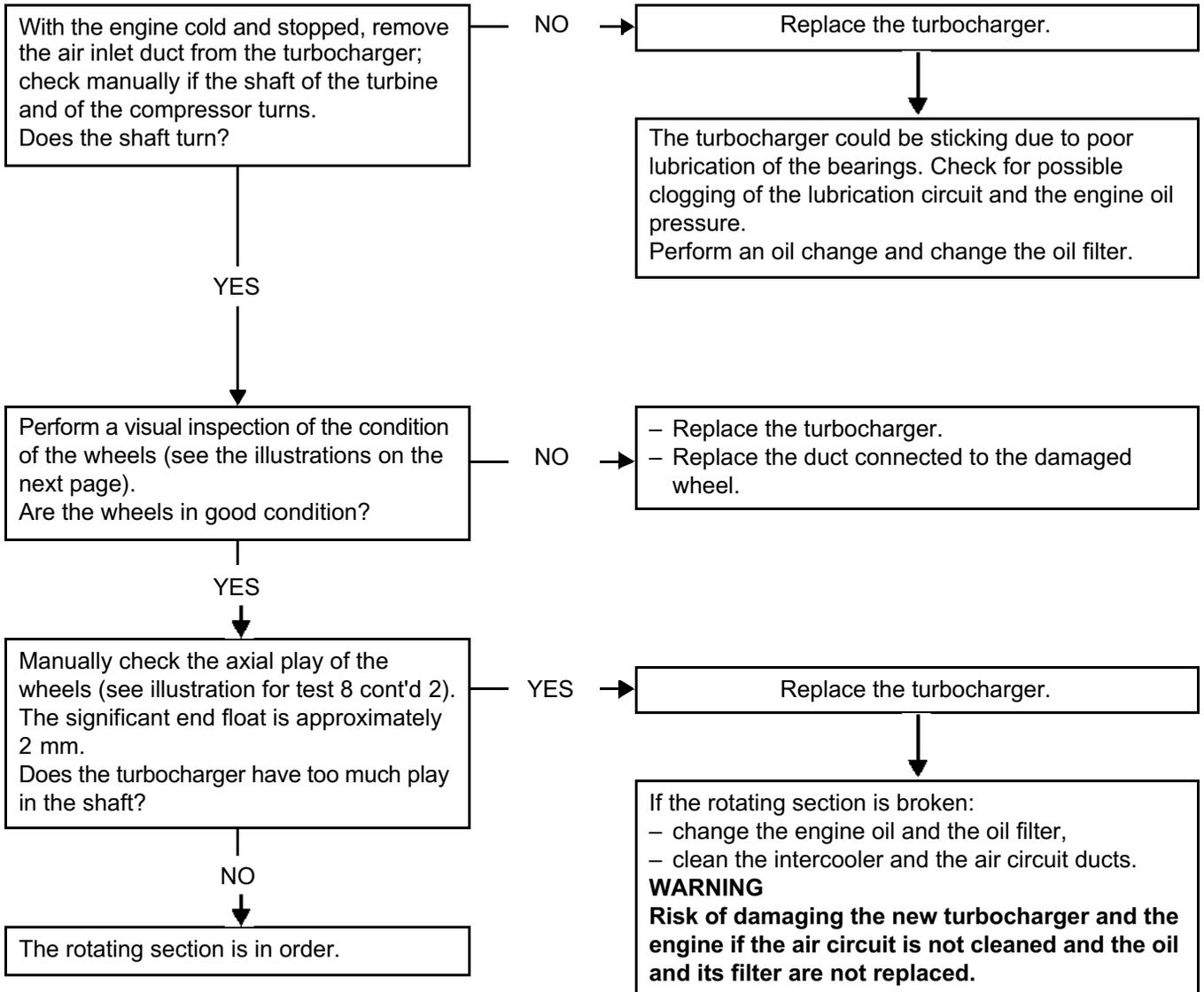
The operating play of the turbocharger bearings is approximately 25 µm (micrometres or microns) between the shaft of the turbocharger and the internal mating face of the bearings and 75 µm between the exterior part of the bearings and the bearing housing.
