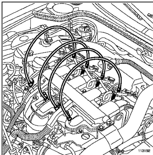
Connect the pipes (3) to the injectors (without removing the clips on the injectors):
