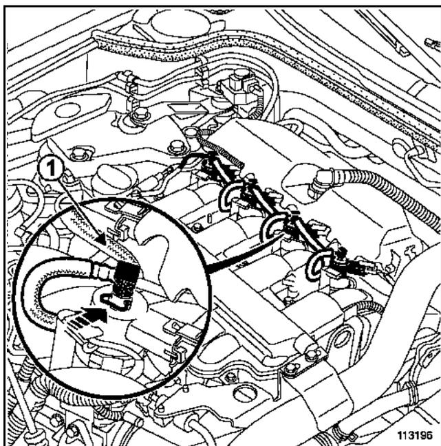
Disconnect the complete fuel return pipe according to the following procedure (do not remove the clips):
