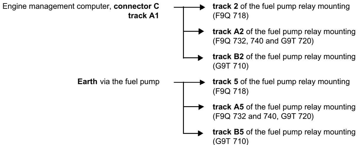
If the fault is still present, change the **fuel pump relay**.
