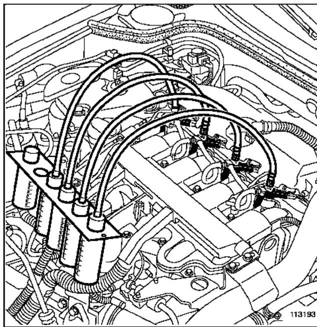
Insert the ends of the pipes into the measuring cylinders of the **Mot. 1760** tool; the cylinders are taken from the **Mot. 1711** tool.
