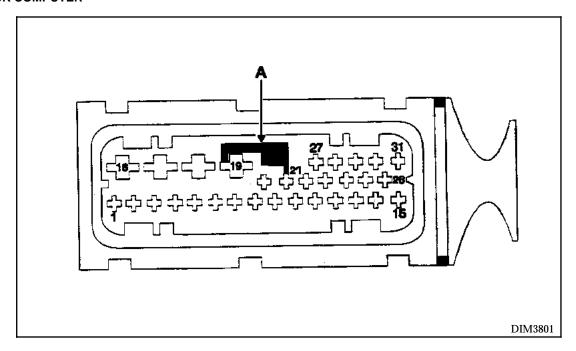
A Micro-spring connecting to earth (terminal 19) and pin 21 (ABS and NIVOCODE warning lights) in case connector is disconnected.
