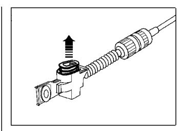
Adjusting the display synchronisation on the instrument panel and the lever repeater.
