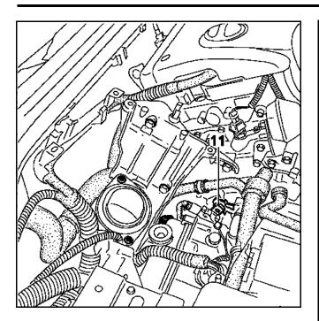
Disengage the sleeve stop by turning the two parts of the sleeve stop in opposite directions a quarter turn (L7X: move the degasser without disconnecting).
