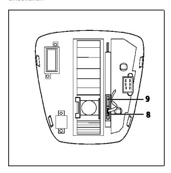
If necessary, place it in high position (refer to the arrow on the diagram below) in relation to the slide rail (9). To carry out this operation, hold the slide (10), attached to the rail between the thumb and the index finger and move the gate with a fine screwdriver.
