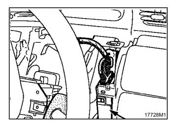
Remove the mounting screws from the central processing unit.
