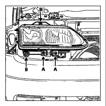
**IMPORTANT:** after refitting the lenses, system initialisation and headlight adjustment must be performed.
