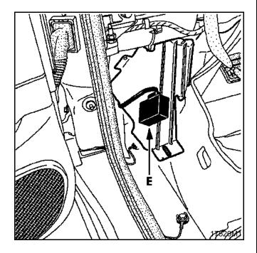
**IMPORTANT:** after replacing the computer, system initialisation and headlight adjustment must be performed.
