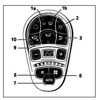
**Note:** In automatic mode (7), remember to close the central air vents on the dashboard when the outside temperature is below a comfortable temperature.
