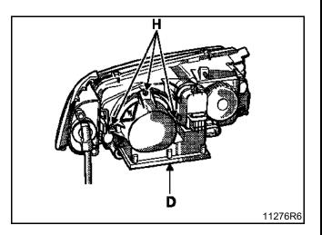
**COMMENT:** the computer (ballast) cannot be separated from the lens unit.
