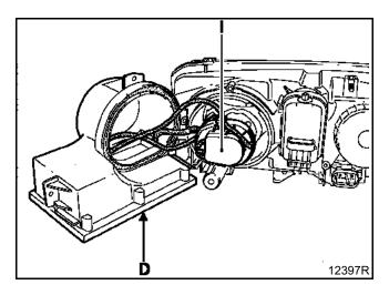
Turn the bulb connector (I) by an eighth of a revolution (anti-clockwise) and release it.
