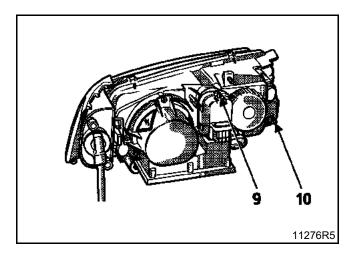
**IMPORTANT:** after replacing the actuators, system initialisation and headlight adjustment must be performed.
