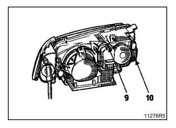
**IMPORTANT:** after replacing the actuators, system initialisation and headlight adjustment must be performed.
