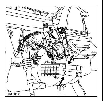
Remove the heater matrices first, then the pieces of pipe.
