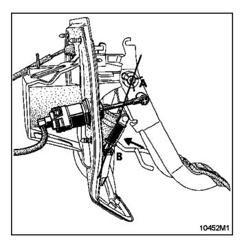
Remove the clutch pedal assistance spring unit; release the pedal and remove the shaft.
