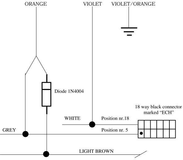
The wire is marked nr.730 located in the wiring harness coming out of the push button inside the driver's side door
