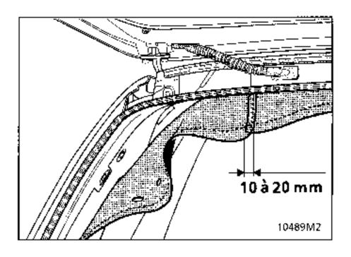
Using a pen, trace out the sewing line (using the original holes) to make fitting easier.
