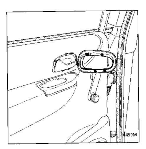
Unclip the door handle surround by lifting the lower section with a screwdriver (TAKE CARE - THIS PART IS FRAGILE).
