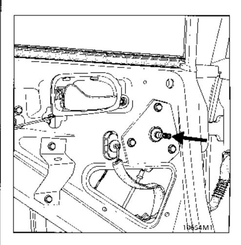
Check the window winder shaft bolt is correctly tightened.
