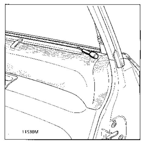
Fit the window winder handle, aligning the handle towards the upper front corner (window closed).
