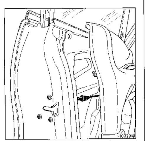
Fit the top of the panel to the inner weatherstrip for the front window.
