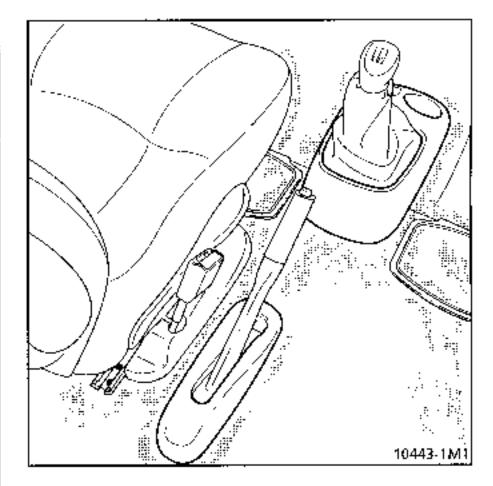
Disconnect the pretensioners and electric seat feeds.
