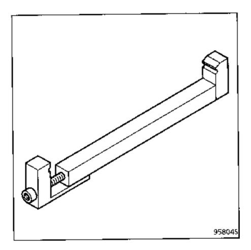
**Car. 1253** tool for removing and refitting the adjusting base strut (front seat base).
