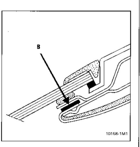
Apply double sided adhesive tape 60 25 109 787 to all the pillar joints and the opening element frames.
