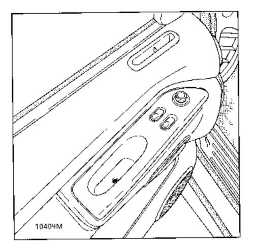
Remove the switch mounting (1 bolt, Torx 20) and release it to the rear.
