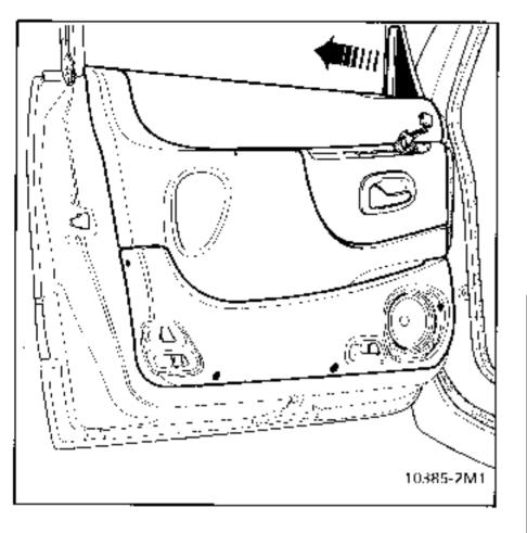
Remove the 4 lower mounting bolts for the storage tray.
