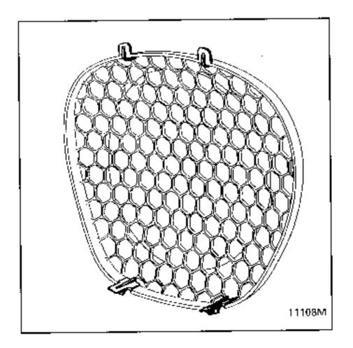
Unclip the speaker grille, releasing the lower section first.
