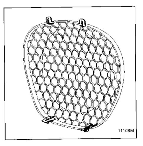
Unclip the speaker grille using a screwdriver, beginning at the lower section.
