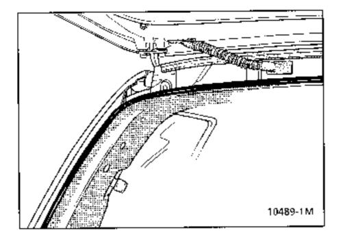
Under the door seals, apply a 19 mm wide strip of black adhesive sealing tape.
