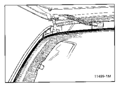
Tighten the lining and bond it onto the double sided adhesive tape.
