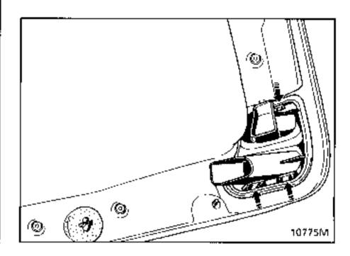
Countersink the 7 welded snap rivets to 6.5 mm.
