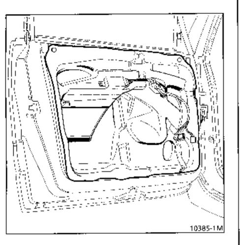
In all cases of removing - refitting the door lining, the sealing vinyl and the preformed mastic bead must be renewed (Part Number : 77 01 423 330).
