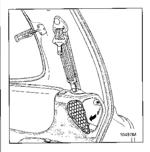
Lift the trim assembly to release the 4 plastic clips at the top.
