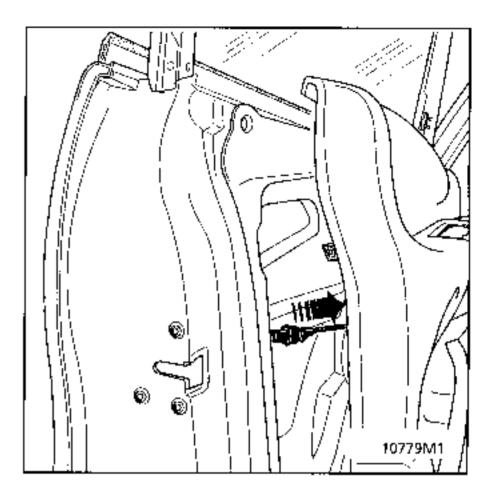
Disconnect the door opening handle on the lock side after sliding the sleeve back.
