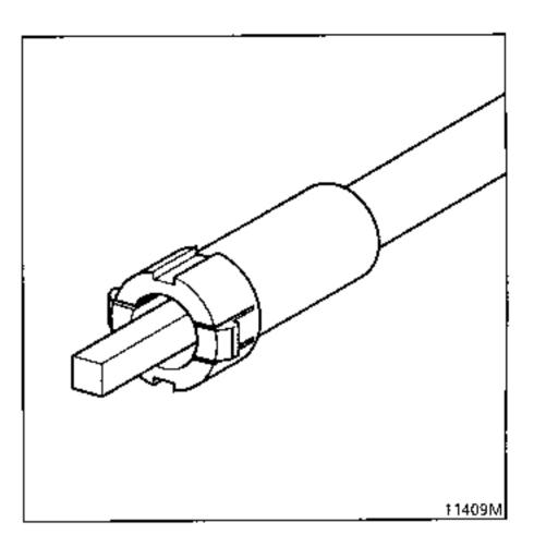
Connect the spindle at the user end by guiding the square drive with a fine screwdriver.
