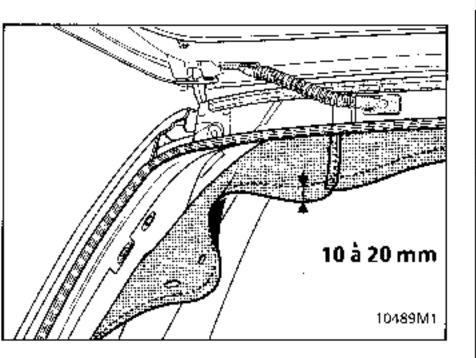
Fit the edging strip (B) between the stretchers and the roof above the front doors, rear doors and the rear quarter panels.
