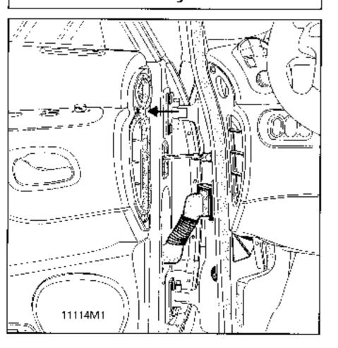
Remove the cover and the bolt in the air inlet duct.
