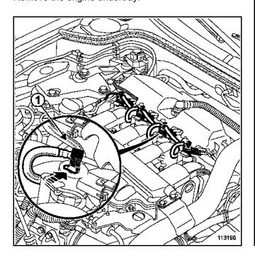
Disconnect the complete fuel return pipe according to the following procedure (do not remove the clips):
