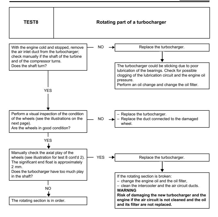
The operating play of the turbocharger bearings is approximately 25  $\mu$ m (micrometres or microns) between the shaft of the turbocharger and the internal mating face of the bearings and 75  $\mu$ m between the exterior part of the bearings and the bearing housing.
