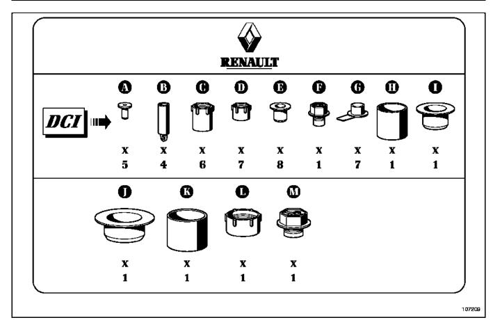
Fit the blanking plugs **(B)**, from the kit (part number **77 01 208 229**), on the end pieces of the fuel return pipe. If fitting of **Mot. 1760** onto the injectors is not being performed immediately, place blanking plugs **(A)** on the injector fuel return openings.
