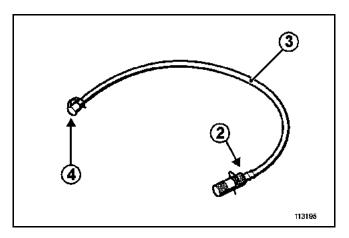
Remove the clips and the plugs from the end pieces (2) of the pipes (3) of Mot. 1760, leave the plugs (4) in place.
